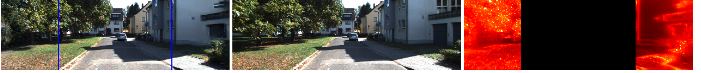
Fig. 1: Given the present and past frames with narrow FoV, we hallucinate the present frame with wide FoV (left: hallucination, middle: ground truth) and predict the associated uncertainty (right). The past frames are omitted for brevity.
